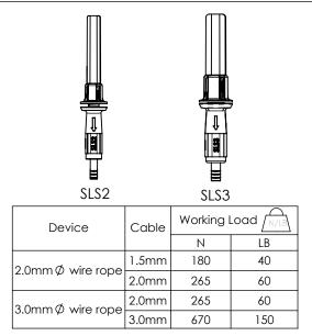
Locking devices are only to be used with nVent CADDY Speed Link wire spools and accessories with the same specified wire rope diameter as the locking device. Do not use with any other wires.
