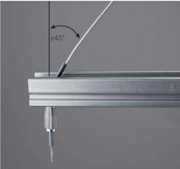
The image above shows the flexibility of the SLS locking device. The device can be installed with a maximum angle of 45°.
