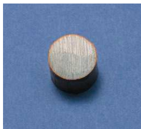
Cu-Bond Round Conductor cross-section
