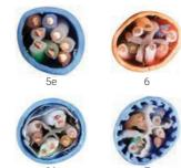
Use higher category cables, which can greatly diminish the impact on temperature. Generally speaking, the temperature rise from category 6A is almost 50 percent less than category 5e. The chart below shows the relationship between temperature rise and current carried by structured cables with bundle size of 25 and exposed cables (rather than those contained in conduit)
