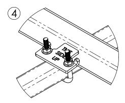
\*Min. Installation Torque: 60 in-lb [6.8 N-m]
