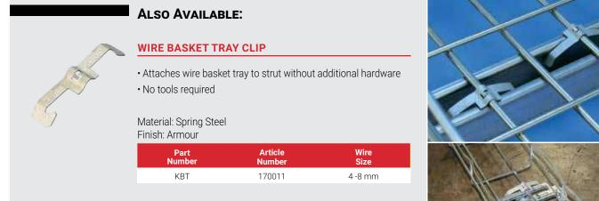
Use two clips per strut support for trays up to 12" (300 mm). Use three clips per strut support for trays up to 18" (457 mm) and add one clip per strut support for each additional 6" (150 mm) of tray width.
