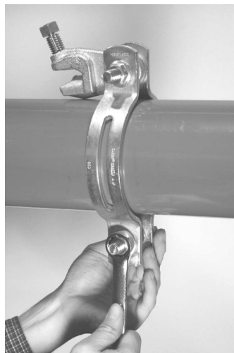
First tighten bolt that passes through brace clamp until the shear head on nut snaps off. Then proceed to tighten the other bolt on the CSBSTU until the shear head on nut snaps off.
