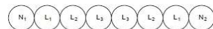
Figure H.52.1 – Special configuration for 6 parallel single-core cables in a flat plane (see 523.7)
