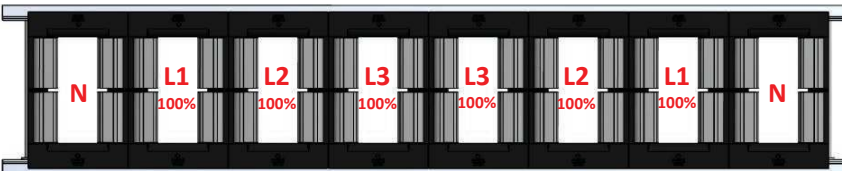
Optimized Conductor Arrangement (Load current balanced)
