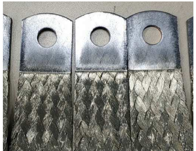
Figure 10 – Close-up shot of the nVent ERIFLEX MJB termination after vibration testing.
