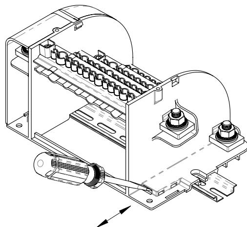
Screw Caps (included) must be used to maintain IP10 rating when larger conductor sizes are installed.
