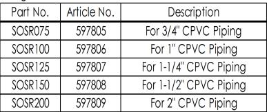
For mounting CPVC sprinkler pipe to the vertical or horizontal face of structural wood, metal, concrete, or composite wood joists with a minimum 3/8" web thickness.
