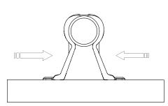
Squeeze strap back around pipe. Note: pipe must be allowed to slide freely.
