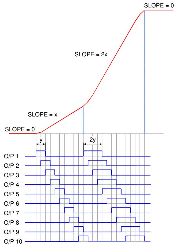
Figure 6: Simplified example of the interleaving principle of the generator. The waveform slope is approximately proportional to the duty cycle.
