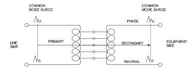
As shown above a transformer provides a path for high frequency common mode transients to flow via capacitive coupling to the secondary with little attenuation.
