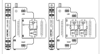
Signal Pair protection, via terminals LINE side 1,2 and EQUIP side 1', 2'. Grounding via ground tab or DIN rail.
