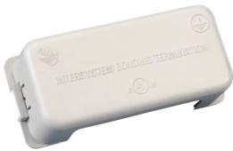
The nVent ERICO Intersystem Bonding Termination Bar is designed to meet rigorous industry standards with options for both zinc and bronze alloy. The Intersystem Bonding Termination Bar is mounted adjacent to the meter base or service entrance equipment, making it convenient to connect and terminate grounding conductors from telephone, CATV, radio, and television antennas. This bar is impact-resistant and UV-stabilized, ensuring durability.
