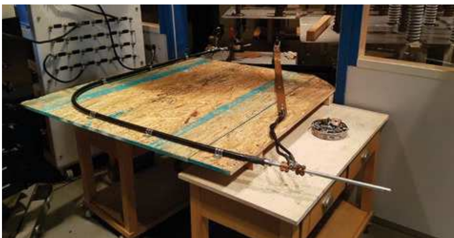
Laboratory testing to verify the 200kA 10/350us rating for the cable with connectors and fasteners
