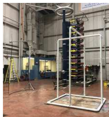
Laboratory testing to verify Equivalent Separation Distance including cable and freestanding mast
