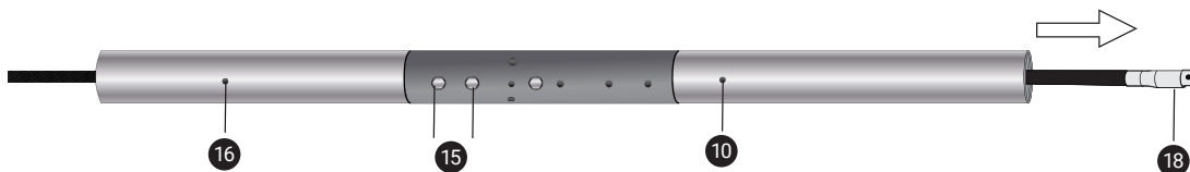
Figure 21—Pass the internal conductor through mast
