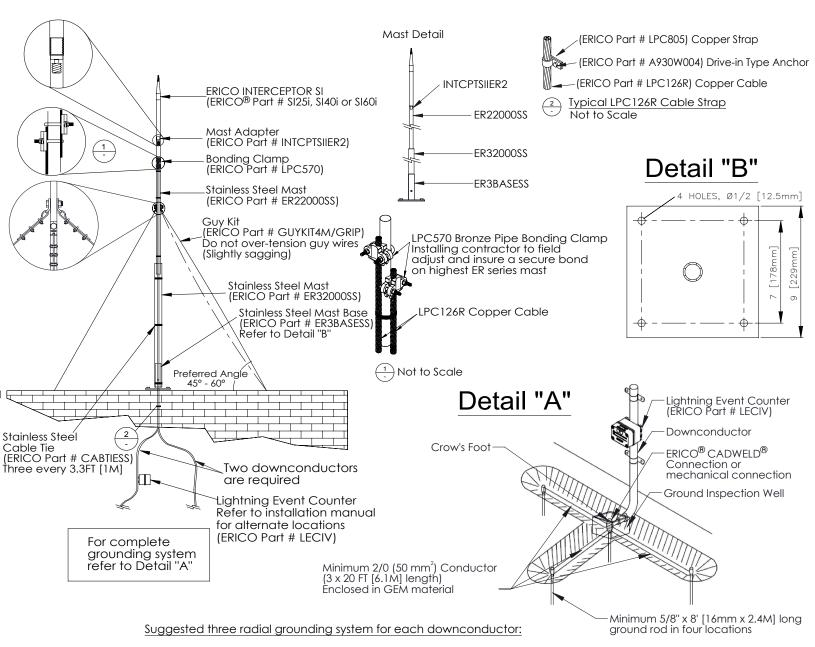
The grounding system shown in the detail is a suggested layout. Each radial consists of a trench approximately 1.5FT [.45M] deep. The conductor is laid in the trench and is connected to ground rods. The conductor in each trench is encased in GEM material. Ground rods must extend 10FT [3M] below ground level.
