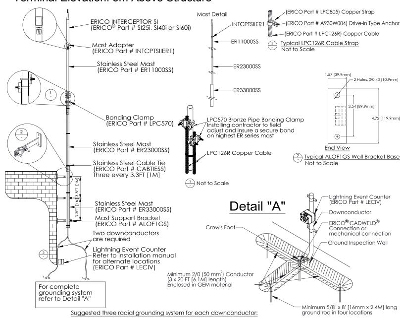
The grounding system shown in the detail is a suggested layout. Each radial consists of a trench approximately 1.5FT [.45M] deep. The conductor is laid in the trench and is connected to around rods. The conductor in each trench is encased in GEM material. Ground rods must extend 10FT [3M] below ground level.
