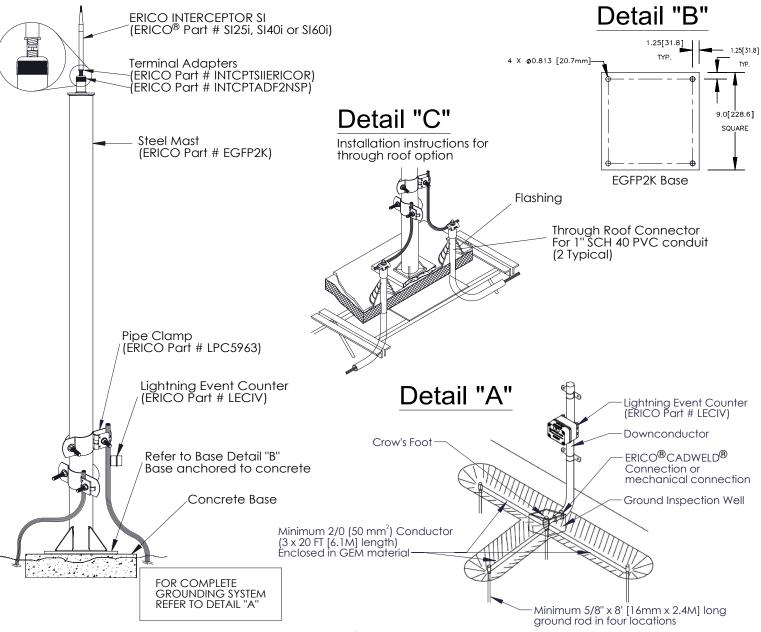
Suggested three radial grounding system for each downconductor:
