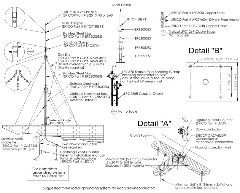
The grounding system shown in the detail is a suggested layout. Each radial consists of a trench approximately 1.5FT [.45M] deep. The conductor is laid in the trench and is connected to ground rods. The conductor in each trench is encased in GEM material. Ground rods must extend 10FT [3M] below ground level.
