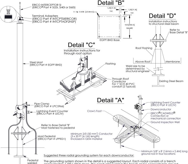
approximately 1.5FT [.45M] deep. The conductor is laid in the trench and is connected to ground rods. The conductor in each trench is encased in GEM material. Ground rods must extend 10FT [3M] below ground level.
