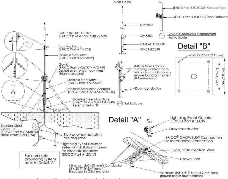
Suggested three radial grounding system for each downconductor:
