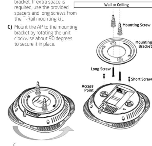
**To attach the AP to a ceiling using T-Rail connectors:**
