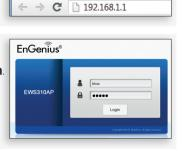
**C)** The EnGenius Access Point User Interface will appear. This device can operate in Access Point operating mode.
