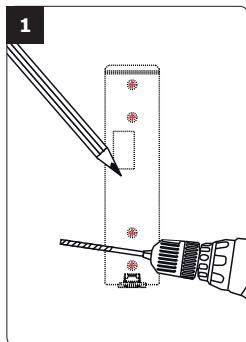
Place the back plate of the PROFIL100EINT on the wall then mark with a pen the hole location then drill the 2 mounting holes (drill bit Ø 5mm and 35mm hole depth) and the hole wiring access.
