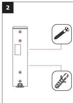
Insert the 2 plastic anchors in the holes. Mount the back plate of the PROFIL100EINT with the screw on the wall.
