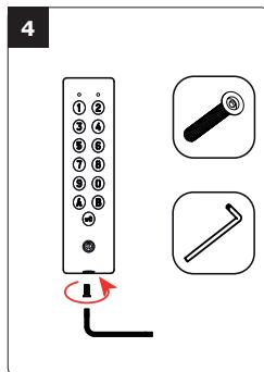
Fasten the PROFIL100EINT keypad to the back plate with the M5x8 Diax® screw and T20 Diax® spanner hardware.
