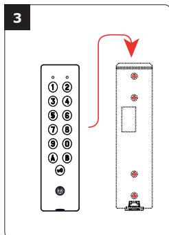
Insert the cable in the hole access area of the back plate. Then mount the keypad on the back plate, placing first the top in the hooks and then the bottom.
