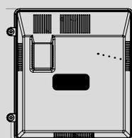
**Position the PSU as follows, with the label placed horizontally.**
