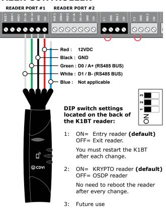
**Note:** Each ATRIUM A22K controller support 2 reader connected in parallel per port (ENTRY and EXIT readers).
