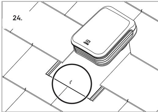
**EN** If the Valetis cannot be placed between two hooks, place the storm spike between two slates. Pierce the flap at the place of the rivet and bend it.
