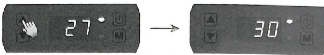
During the heat pump unit running, press the Increase/Upwards button or the Decrease/Downwards button to set the required temperature.
