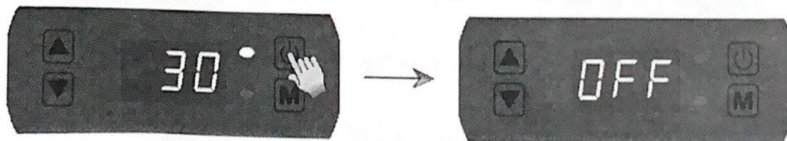
Push the On/Off button to stop the heat pump unit. The heat pump unit will shut down, but the fan will keep on turning for 30 seconds.
