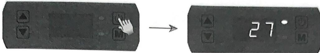
When the heat pump unit is under standby, push U the On/Off button to start the unit. The current entering water temperature will appear and the heat pump unit will start automatically. When the inlet water temperature is lower than the setting temperature, the unit will run under heating mode, and the heating indicator (Red) will be active.
