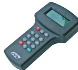
The service unit is used to provide power to the safe in the event the safe battery is flat, to override (unlock) the safe in the event the user code is forgotten and to access the log of the last 200 operations.
