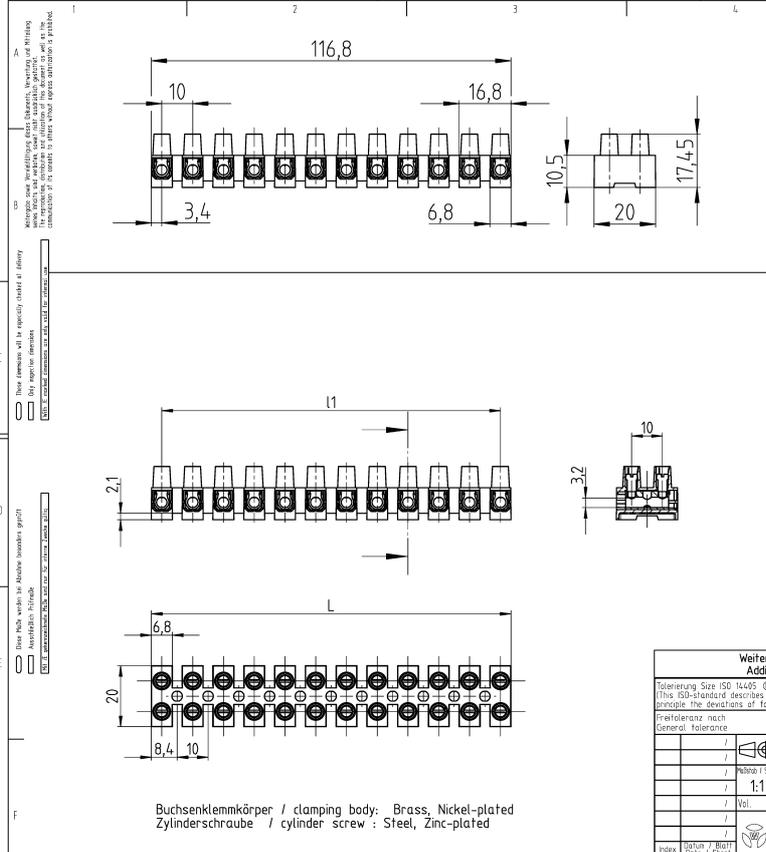
Buchsenklemmkörper / clamping body: Brass, Nickel-plated
