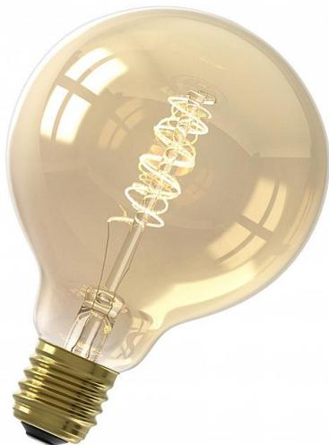
**LED Flex Fil G95 E27 DIM 3.8W (25W) 250lm 2100K Or**
