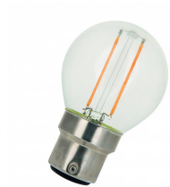
145333 LED FIL G45 B22d 12V-24V AC/DC 2W (21W) 200lm 827 Clair
