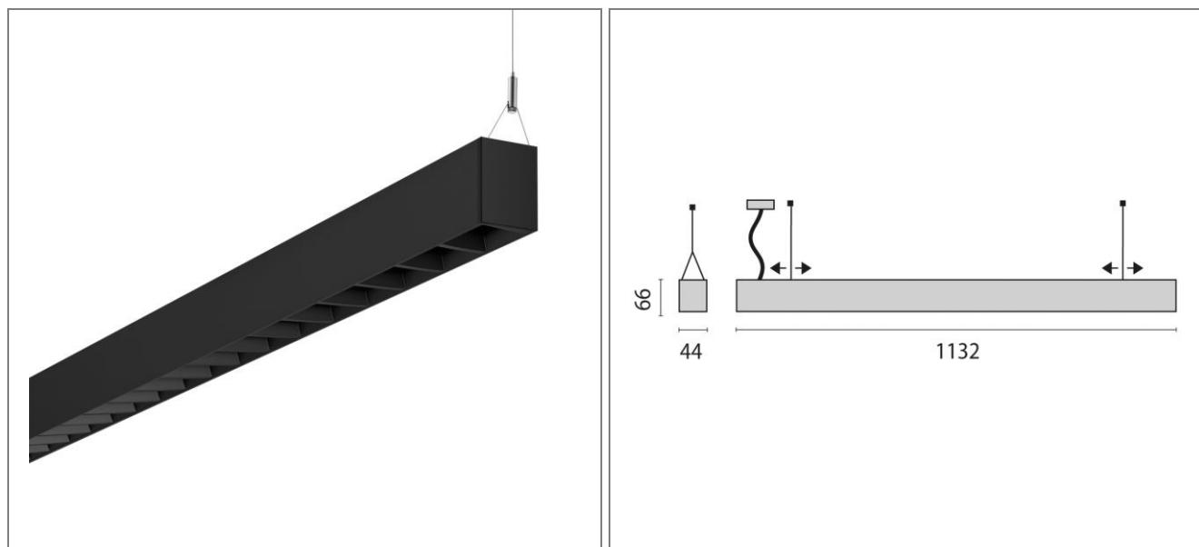
Art.: 3112561, SL764+ PL M 36 S/B 840 BK9005 LV, Suspended, LED luminaire for indoor, comprising: Extruded aluminium profile housing, die-cast aluminium end caps, painted. Black grid for maximum luminaire efficiency, glare reduction and a high uniformity. Streamlined, simple design with flush end caps. High-quality workmanship of profile connections for a perfect look. High economic efficiency thanks to luminaire efficiencies of up to 155 lm/W.
