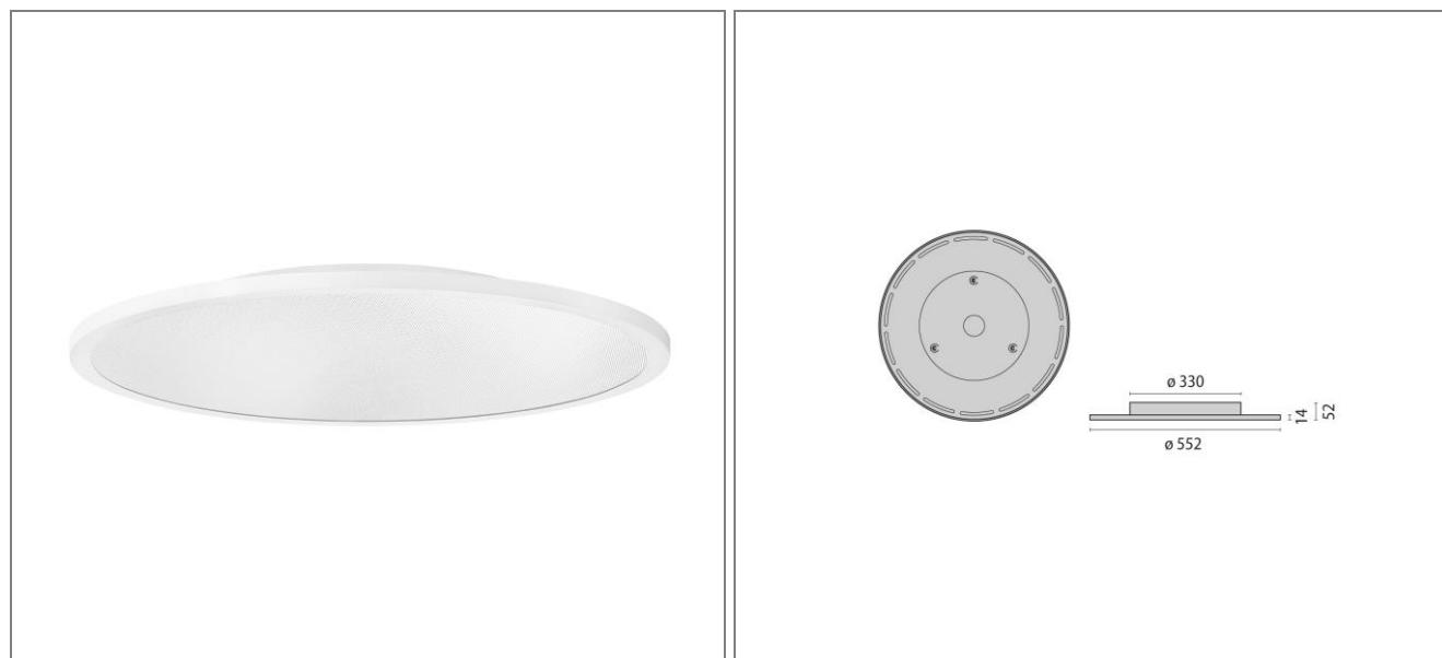
Art.: 8555661513310, FL ROUND 555 AB, Direct/indirect, 50W, 3000K, Driver static, 552mm, Symmetrical, > 75°, White, Wall and ceiling mounted LED luminaire for indoor, comprising: Housing made from sheet steel and diecast aluminium, powder coated. Micro-prismatic diffuser for efficient light diffusion, glare reduction and a high uniformity. LED Sidelight-Technology and light orienting plastic optic for a homogenous light distribution over the entire area of the diffuser.
