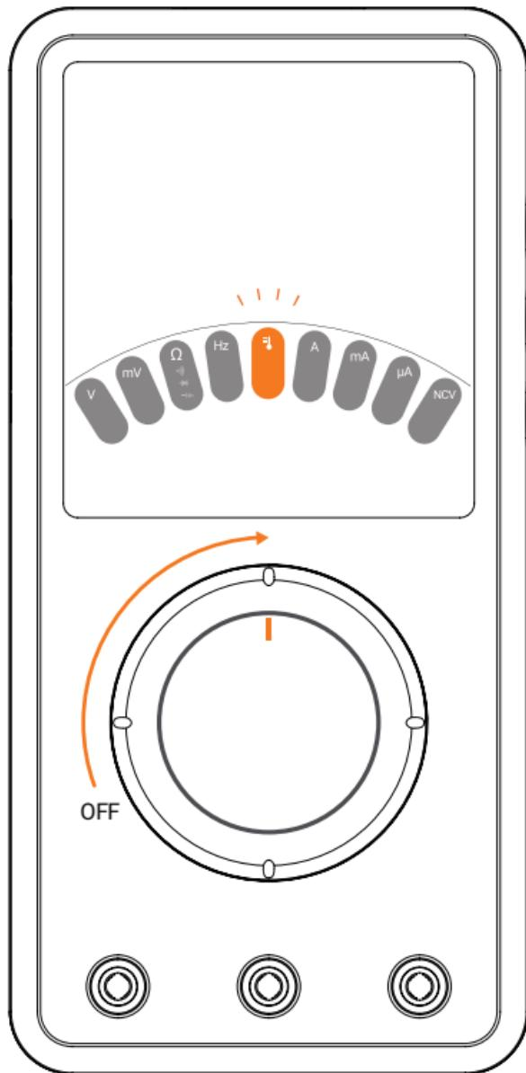
Set the desired measurement by turning the rotary dial. The position of the dial will be shown on the display. Power off the Multimeter by positioning the dial to OFF at the counterclockwise end position. The functions of the dial positions are as follows:
