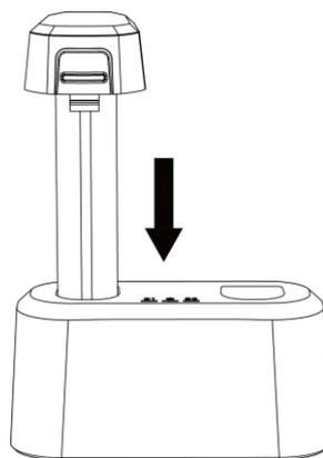
**Figure 2-7 Charge Battery**
