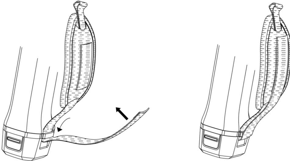
Figure 2-2 Secure Lower Part of Hand Strap
