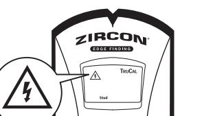
**WARNING** Electrical field locators may not detect live AC wires if moisture is present in the wall, or if wires are more than 50 mm from the scanned surface, in plastic conduit or behind a plywood shear wall or metallic wall covering.
