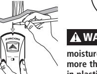
Without releasing Power button, continue scanning beyond marked spot until some segments of the arrow turn off. Slide unit in reverse direction to locate other edge of stud.
