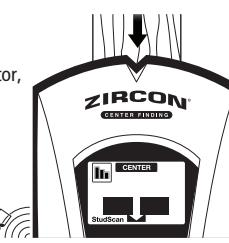
In cases of deeper studs (thicker walls), when the centre of the stud is located, only two bars will show on the Signal Strength Indicator and only the SpotLite® Pointer and middle segments of the Target Indication Bars will illuminate. If you still cannot locate a stud, try DeepScan® mode. Display will light green with the word "DeepScan" to indicate the mode.
