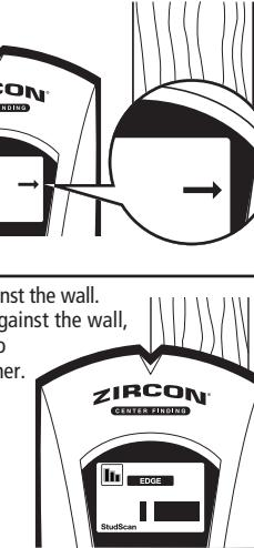
Continue sliding the tool. When the centre of a stud is located, the three bars on the Signal Strength Indicator, the middle segments of the Target Indication Bars, CENTER indication, and SpotLite® Pointer will all illuminate and the buzzer will sound.
