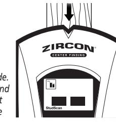
*Note: To determine if the object located is a wood stud, metal stud, or pipe, scan the location in Metal Scan mode. In Metal Scan, only the metal drywall screws will be found in wood studs, while metal will be indicated throughout the entire metal stud or pipe. To better determine if the target object is a metal stud or pipe, studs usually run floor to ceiling whereas a pipe may not.*
