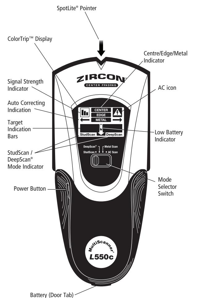
Make sure your fingertips are resting on the handle and not touching the surface being scanned or the scanning head of the tool.
