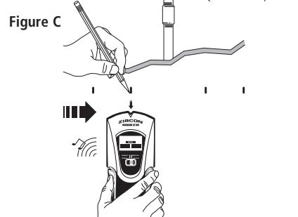
narrow the scan area. This procedure can be repeated multiple times to narrow the scan area even further (Figure C).
