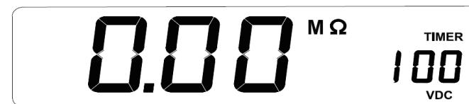
Press SELECT to check the preset time. The LCD screen display TIMER, PRES is shown on primary display, the secondary display shows the preset time. Press ENTER, the meter display Set. The time can be adjusted by  $\Delta/\nabla$  button. Presss ENTER again to confirm the adjustment.
