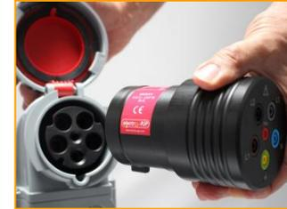
The markings and the colors of the banana female connections show me where to connect to the phases, the neutral, the protective earth, and the pilot.
