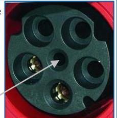
Of course the pilot conductor is useful providing that it is integrated in an electric circuit made to switch off the load. So the adapter offers a safety 2 mm banana connection which is mated to the center pilot pin of the adapter. By connecting a 2 mm banana plug to the safety 2 mm banana female connection it is possible to connect to the switching electric circuit or to make another one.
