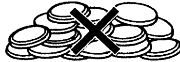
Example of stacked and jumbled batteries
