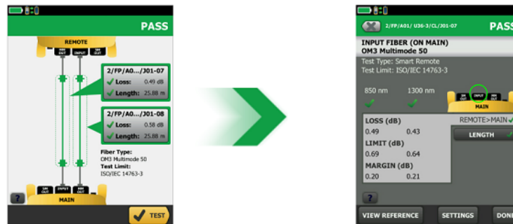
Complete data is displayed with a test result. The dotted line shows what's included in the measurement. Detail windows show the results for each fiber tested.
