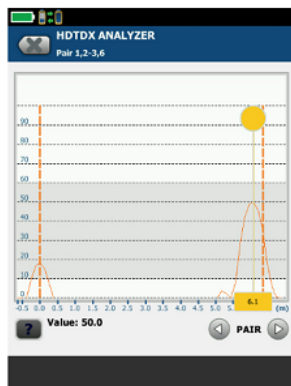
High Definition Time Domain Cross talk (HDTDX) shows the far end connection is clearly the issue
