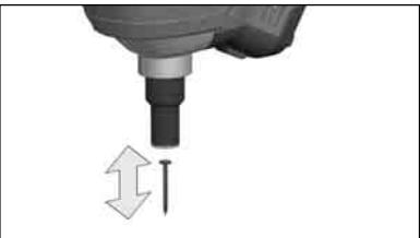
Nails with very small heads (< 5 mm) or broken heads could get jammed. Pull jammed nail with a pliers or unscrew the collet.
