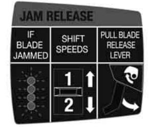
If blade jammed all fuel gauge LEDs will blink. Move the speed control switch between „1“ and „2“ several times back and forth. Pull the blade release lever.
