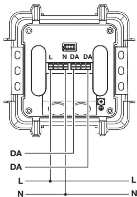
The power supply line consists of a 4- or 5-core cable:
