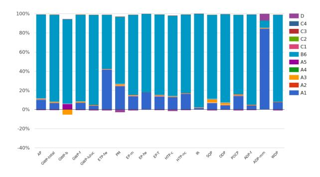
Luminaires are products that consume energy in the form of electricity during the usage phase. This has the highest impact on the environment during the product's long service life. The actual impact in B6 depends on the usage scenario, luminaire settings and the energy mix. The impact can therefore vary depending on the usage scenario.
