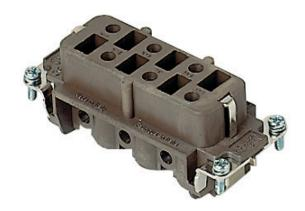
Female insert, CP RY series, screw terminal connection, 6 poles + PE, 35 A 400/690 V 6 kV 3, size "77.27", for applications up to 180°C, with plate
